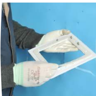
Place the seal over the flange
